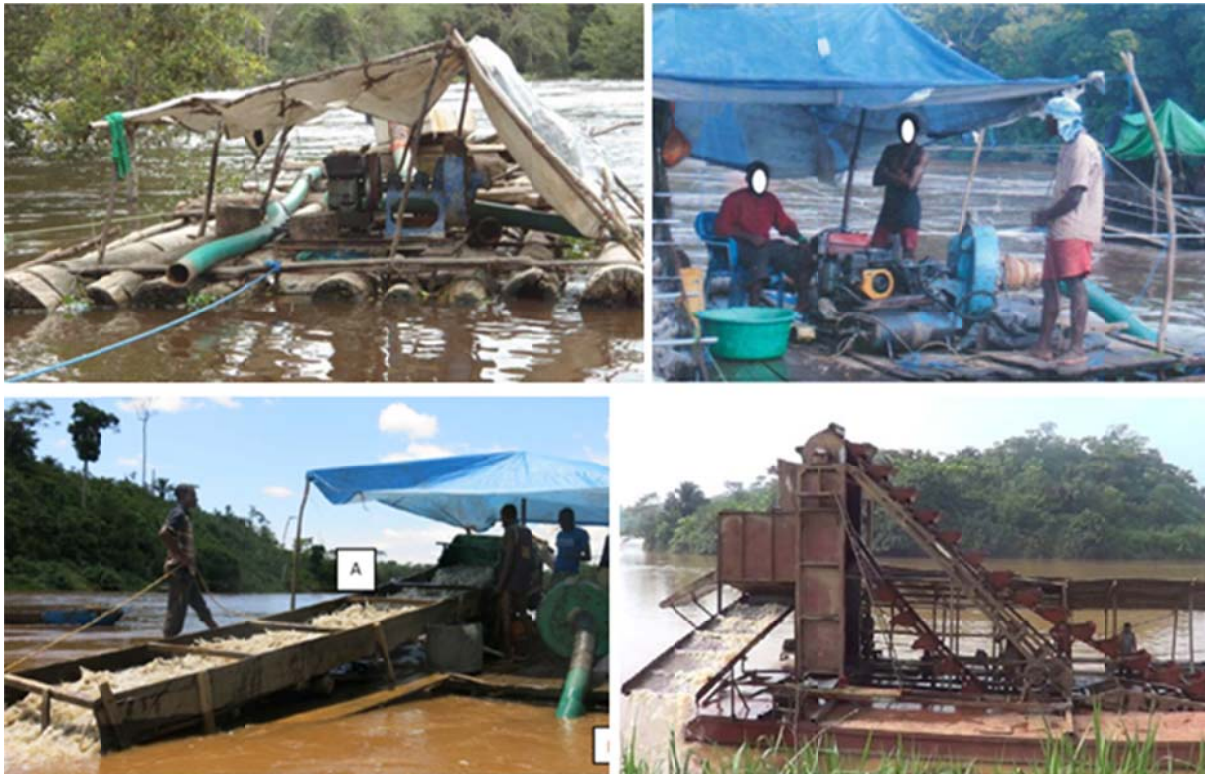
Figure 18: Gold dredges in the DRC, suction dredges [Top left - Gangu River (IPIS 2012), Top right - Osoo River (GoE 2014), Bottom left – Ulindi river (COSOC 2015)] and bucket line dredge [bottom right – Ulindi river (COSOC 2015)].
