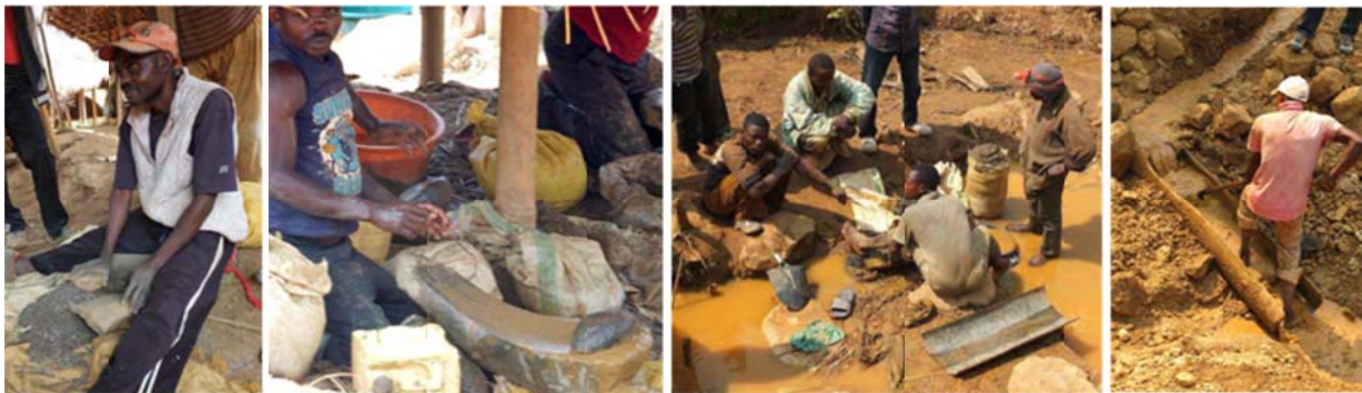
Figure 16: Crushing, grinding and washing at different ASM sites, source: ARM (2014b).
