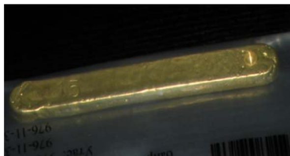
Figure 10: ASM doré bar, assayed and sealed for legal export. Source: F. Hruschka.
