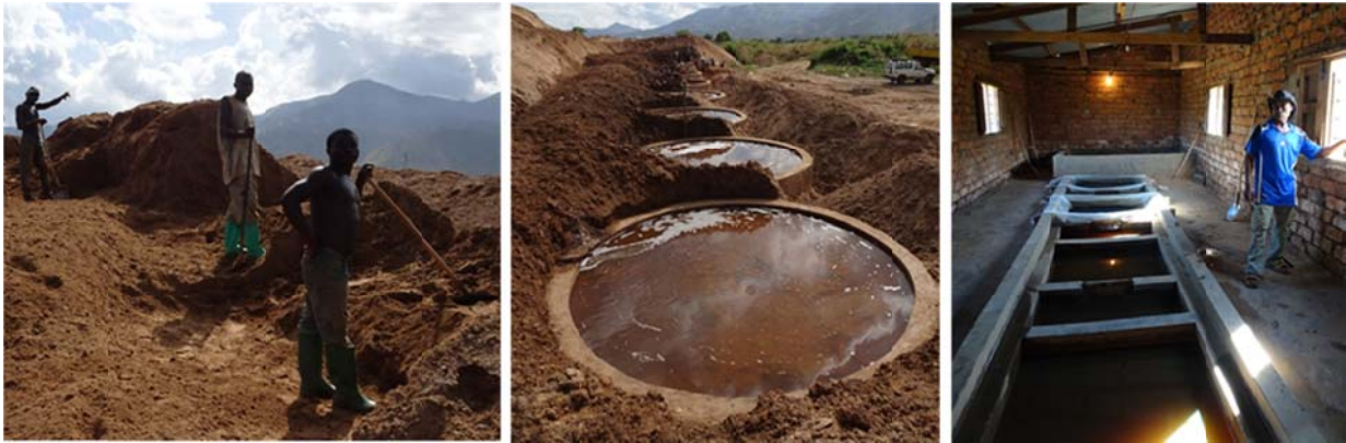
Figure 17: Small-scale cyanide leaching plant in Misisi / South Kivu, source: D. Ruppen.
