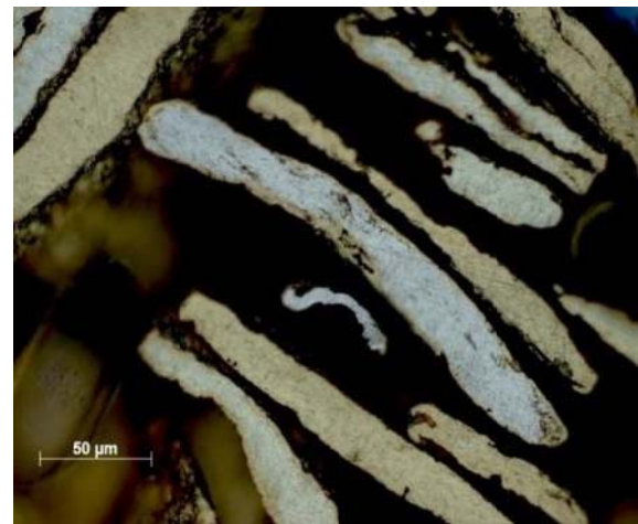
Figure 6: Native gold as flakes. Silver rich gold is whitish, whereas silver poor gold is yellowish, Rheinzabern, source: T. Oberthür.
